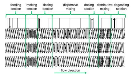
**Figure 2.**Screw configurations used in the experimental setup.
