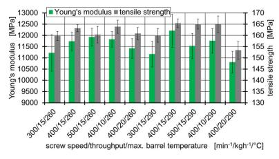
Figure 3. Young's modulus and tensile strength for different process parameters at a maximum barrel temperatures of 260 and  $290\,^{\circ}$ C.
