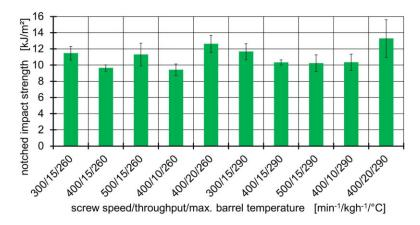
**Figure 4.** Notched impact strength for different process parameters at a maximum barrel temperatures of 260 and  $290\,^{\circ}$ C.
